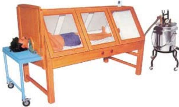
Lying Steam-Bath, hardwood constructed, with three glass windows, on each side. Steam is generated by 2 Kw. electric boiler with safety devices. The steam passes in the box from both sides & can be controlled by gate valves. A special moving trolley with perforated bed, where patient lies, is an integral part of the unit. Fitted with dial thermometer.
