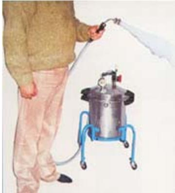
Suitable for giving steam bath at a particular point. The aluminium body boiler is fitted with an electric heater, pressure gauge, safety pressure valve, steam flow control valve and a pointed nozzle to give proper steam-bath at a point.
